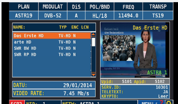
Measuring the current video data rate of "Das Erste HD" with image display
