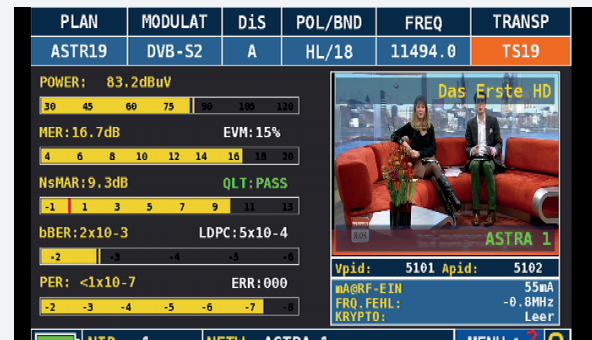
Clear display of level, MER, noise margin, bit error rates and associated live image
