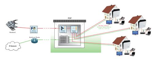
**Ethernet Point-to-Point Topology (EPTP) One-Fiber-Solution**
